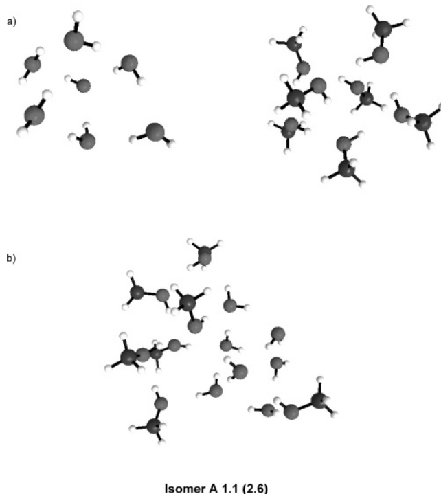
Figure 11. (a) Lowest energy isomers for (\text{MeOH})_7 and (\text{H}_2\text{O})_7 clusters; (b) the lowest energy isomer from MC/SA initiated from 7\text{MeOH} + 7\text{H}_2\text{O} \sim 5 \text{ \AA} apart; EFP2 (MP2//6-311++G (2d,2p)) (kcal/mol).
